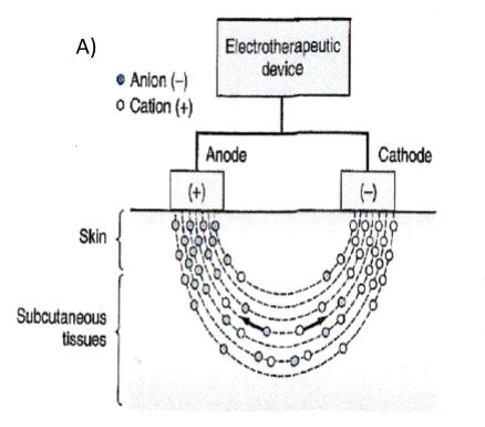
Electrons flowing from the electrotherapeutic device through the lead wires to the electrodes on the patient, inducing ion flow in the biologic tissues beneath the electrodes.
